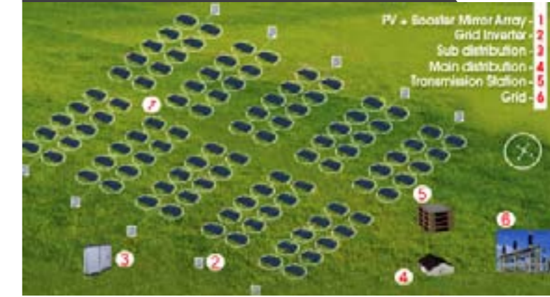
On Grid Solar Field
